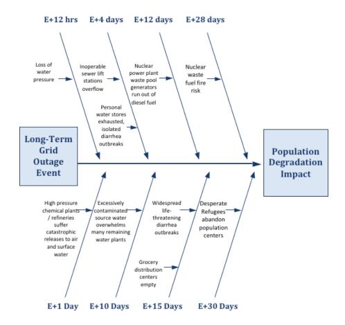
Fig. 1. Long-Term Power Outage Worst Case Timeline, as shown in *Powering Through*, p. 166 (Source: Stephen Volandt, Auroros Incorporated).
